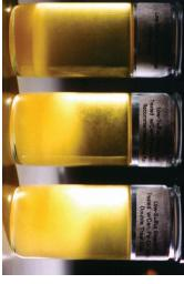
point for 12 hours. \*Static state diesel fuel test at 10°F below cloud
